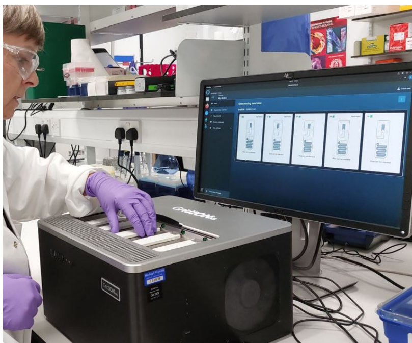
Figure 3. Long-read sequencing Oxford Nanopore platform used for deciphering the genome of black rice landraces.
